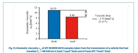
The ATF viscosity tests were carried out at a temperature of 80 °C corresponding to the normal working temperature of the AT under tests. Pursuant to Polish Standard PN-EN ISO 3104:2004, the ATF viscosity shall be determined at temperatures of 40 °C and 100 °C [14]. In authors' opinion, however, the measurements of fluid viscosity at a temperature of 80 °C could help to identify the reasons for malfunctions of the automatic transmission under tests.
