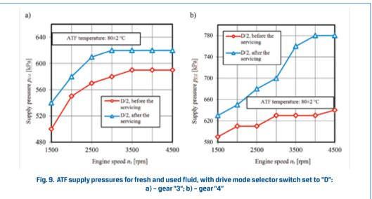
After the servicing, the actuator supply pressure  $p_{\scriptscriptstyle DI}$  for the transmission operating in gear "3" changed from  $p_{DI}$  = 560 kPa at an engine speed of  $n_s$  = 1500 rpm to  $p_{DI}$  = 620 kPa at an engine speed of  $n_{\rm e} = 4\,500$  rpm, i.e. these pressure values exceeded the corresponding figures recorded before servicing the transmission by 10.7 % at  $n_c$  = 1500 rpm and by 4.84 % at  $n_s = 4500$  rpm.
